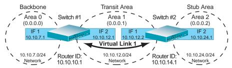
Figure 4-6 Configuring a Virtual Link
